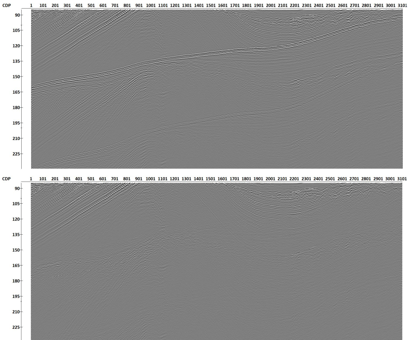
Stacks before (top) and after (bottom) Zero-Offset DeMultiple-based multiple subtraction
