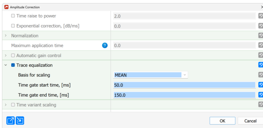
Amplitude Correction parameters for trace equalization
